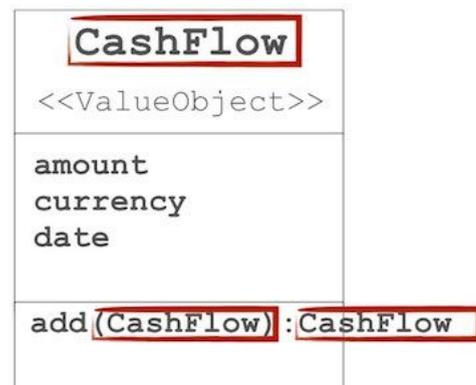
Looking at the UML class diagram, it's striking that the class only refers to its own type, or primitives (in the constructor, not shown here). Methods take Cashflow as parameter, and return Cashflow, and nothing else.
